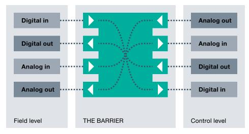
THE BARRIER adapts oneself to the required signal type - no configuration necessary!
